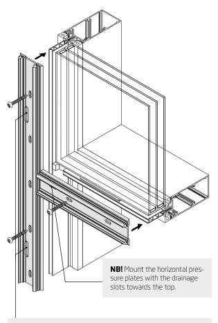
**NB!** Always mount the vertical pressure plates with the ventilation slots facing the same side of the screen.
