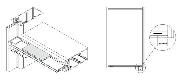
Step 2. Place door/window into the opening. While using glass adjustment tool, unify distance between frame and façade section all around.
