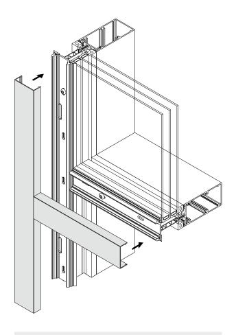
**NB!** Drainage openings in decorative profiles should always be positioned towards bottom.
