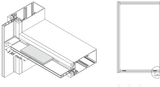
Spacer distance plate shall cover the whole glass edge.
