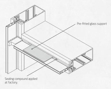
· Windows/doors arrive with preassembled add-ons, prepared for installation in to the openings of the façade.
