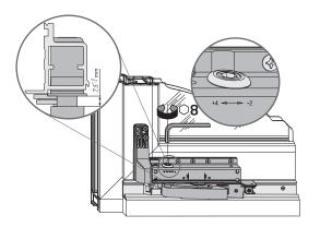
Adjustment of the height position of the parallel slide & tilt element
