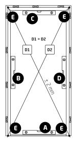
Frame jambs must be square and plumb in both directions and the diagonals (D1 and D2) should be identical.
