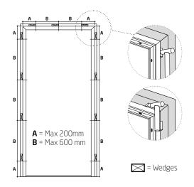
**Step 1.2** Fix the frame with wedges. Wedges must be positioned next to each fixing point on the doorframe.
