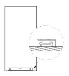
**Step 1.1** Prepare the opening for installation. The entire base under threshold must be flat and level.
