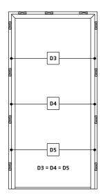
Check the rebate widths are equal across the hinge and locking points (D3,D4 and D5).
