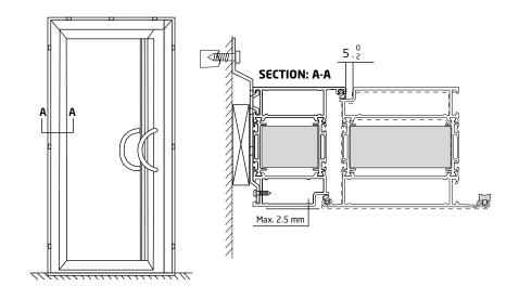
**Step 3.7** If door is produced with smoke protection class Sa/S200, Please follow maximum height limitations between door leaf and threshold/floor. Adjust if needed.
