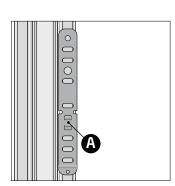
**Step 1.1** Bracket should be fitted in one line of the profile. Bracket "knobs" should be fitted in the grooves (A)
