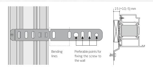
**Step 3.2** Fasten the door with the screws of steel to the wall.
