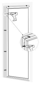
**Step 3.3** Ensure horizontal and vertical levelling of the frame (according to Step 2.3).
