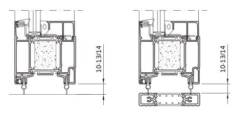
**Step 3.8** Adjust top secure pins M4x16. Check the functionality of sash. Adjust if needed.
