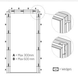
**Step 2.2** Fix the frame with wedges.
