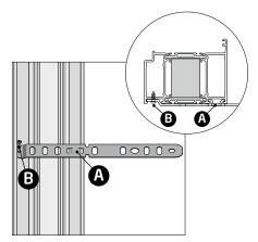
**Step 1.3** The bracket should be fastened to the frame with screw (12165). One pc./bracket (B).
