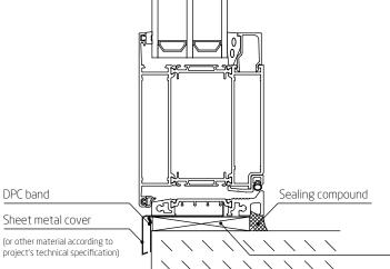
**NB!** If it will be decided to use bearing support beneath the threshold it must be in level and continuous end-to-end.
