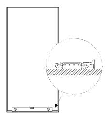
**Step 1.1** Prepare the opening for installation. The entire base under threshold must be flat and level. If it will be decided to use bearing support beneath the threshold it must be in level and continuous end-to-end.
