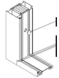
Plastic cap has to be sealed with sealing compound for fire rated doors P/N 12222. Applies to external constructions only.
