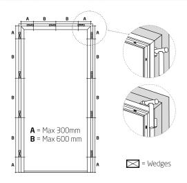
**Step 1.2** Fix the frame with wedges.
