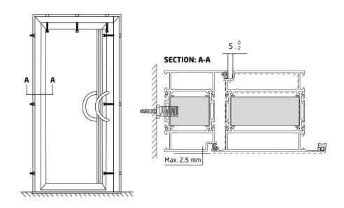
**Step 2.7** If door is produced with smoke protection class Sa/S200, Please follow maximum height limitations between door leaf and threshold/floor. Adjust if needed.
