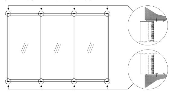
**Step 2.** Ensure horizontal and vertical leveling of the profiles.
