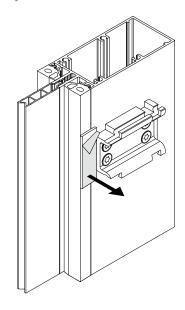
**Step 2.** Fit transom on the bar cleat, pre-compress the joint by clamping before fitting the screws. Release the end of the gasket.
