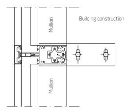
Fixation at side. Postion and type of screw must allow thermal movement.
