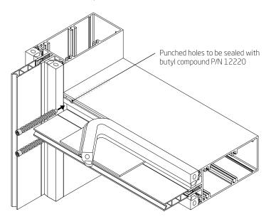
**Step 4.** Insert rebate filler between transom and mullion. Rebate filler is supplied with the order. Rebate filler must be sealed with butyl compound P/N 12220.
