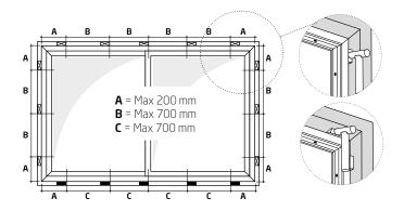
**Step 5.2** Fix the frame with wedges into the wall opening. The wedges must be positioned next to each fixing point on the frame.
