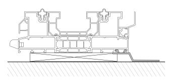
**Step 5.5** Ensure horizontal and vertical leveling of the frame.
