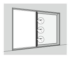
**Step 3.3** Remove the glazing beads from the fixed part. Push the glazing bead forward in order to free up and place it safely.
