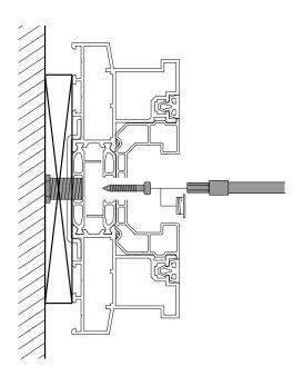
**STEP 6.2** Screw bolts through brackets.
