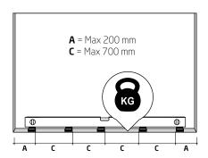
**Step 5.1** Place bearing pads at the bottom of the opening next to each fixing point on the door. The number of bearing pads must correspond to the number of fixing points. Ensure they are level.
