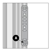
**Step 4.1** Bracket should be fitted in one line of the profile. Bracket 'knobs' should be fitted in the grooves (A).
