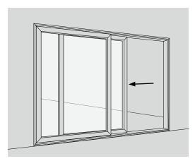
**Step 2.2** Lift the sash up and tilt the bottom against the frame. Take the sash out.
