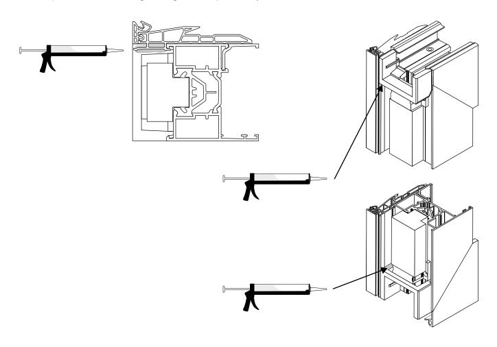
**STEP 8.4.** Apply silicone in the grove of the aluminium cover (A). Fit it back to the place (B).
