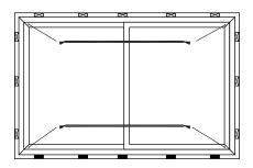
In the case of wide frame profiles, the top and bottom frame leveling can be checked by using a laser or string.
