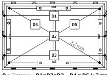
**D** = Distance **D1=D2=D3 D4 = D5 (±2 mm)**
