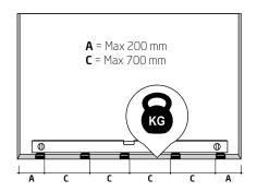
**Step 2.1** Place bearing pads at the bottom of the opening next to each fixing point on the door. The number of bearing pads must correspond to the number of fixing points. Ensure they are level.
