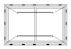
In the case of wide frame profiles, leveling of the top and bottom frame can be checked by using a laser or string.
