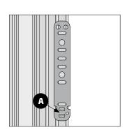
**Step 1.1** The bracket should be fitted in one line of the profile. Bracket 'knobs' should be fitted in grooves (A).
