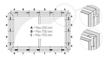
**Step 2.2** Fix the frame with wedges into the wall opening. The wedges must be positioned next to each fixing point on the frame.
