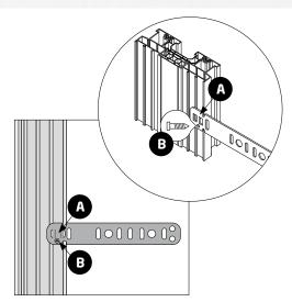
**Step 1.3** The bracket should be fastened to the frame with a screw. One pc/bracket (B).
