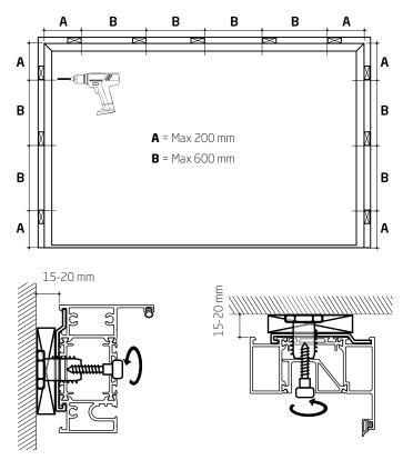
**Step 2.1** Screw bolts through the adjufix sleeves on the frame. The recommended distance and depth of drilling according to the type of the wall is shown in the scheme to the right. Cover the pre-drilled holes with caps for finishing.
