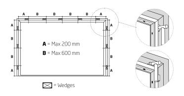
**Step 1.3** Fix the frame with adjufix sleeves into the opening. Open the sash and support it while fixing the frame to the opening with the help of the hexagonal screwdriver bit.
