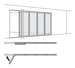
$\textbf{4.} \ \ \text{Finish by closing the main sash and locking it with handle No} \ 1.$
