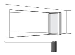
**6.** The folding door is completely opened and is held by the magnets.
